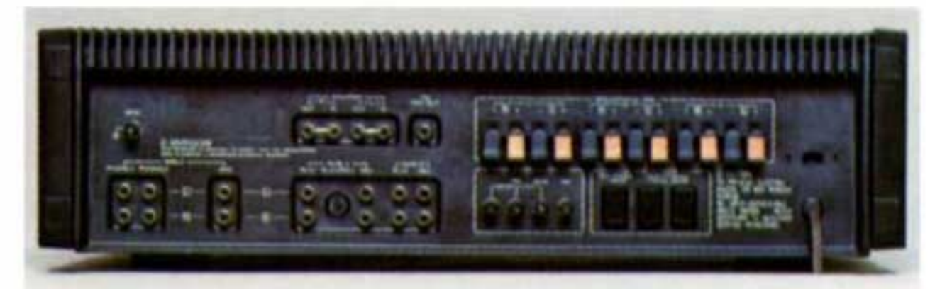
Recessed rear panel for complete cable protection
