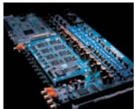
4-Layer DSP Processing Board in the DSP Chamber
