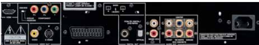
The DVD-S2500 rear panel offers optical and coaxial digital audio output terminals, component video output terminals (progressive/interlace), S-Video and composite video output terminals, mixed 2-channel audio output terminals, 5.1-channel discrete audio output terminals, HDMI terminal, dual i.LINK (IEEE1394) terminals, RS-232C interface, remote control IR code input/output, a terminal for a detachable power cable and SCART terminal.
