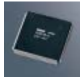
YGV-619 video processor LSI (Yamaha original)
