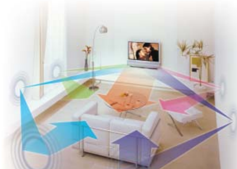
Sound is projected at the listener from five directions: straight ahead, reflected off one wall, and reflected off two walls (so it is heard from the rear).
