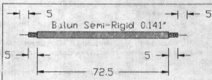
Figure/Abb. 3: Semirigid Balun
