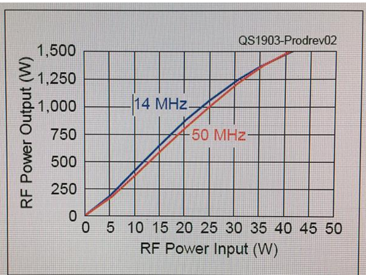
Figure 2 — Elecraft KPA1500 RF input power versus output power.
