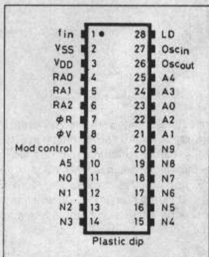
Fig 1: Pin connections for the MC145152-P2.
