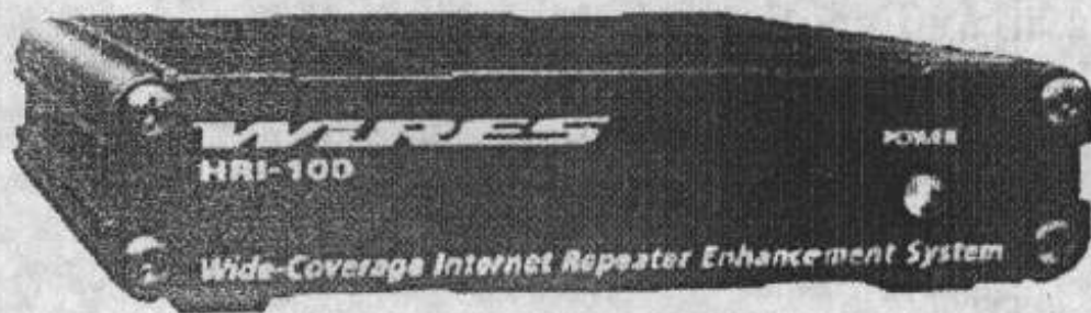
Figure 4—The hardware controller at the heart of the Yaesu WIREs-II system.
